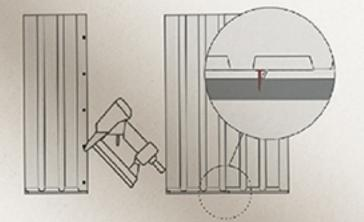
5 When joining panels on the corner of the wall, groove the panels together.
