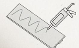
The panels can be installed vertically or horizontally. In addition to the mounting glue, you can additionally use a stapler to attach the panels to the wall. Apply the staples to the edge of the panels' tongue, making them invisible.
