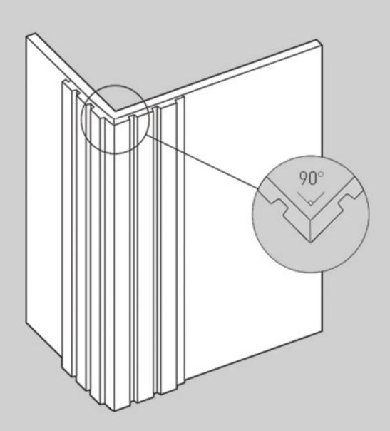
The panels can also be installed in the corner according to the diagram below
